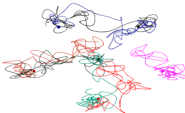
Figure 11. Trajectories followed for every atom in the \text{Na}_7 cluster projected on the equatorial plane in a period of 8 ps at 300 K.
